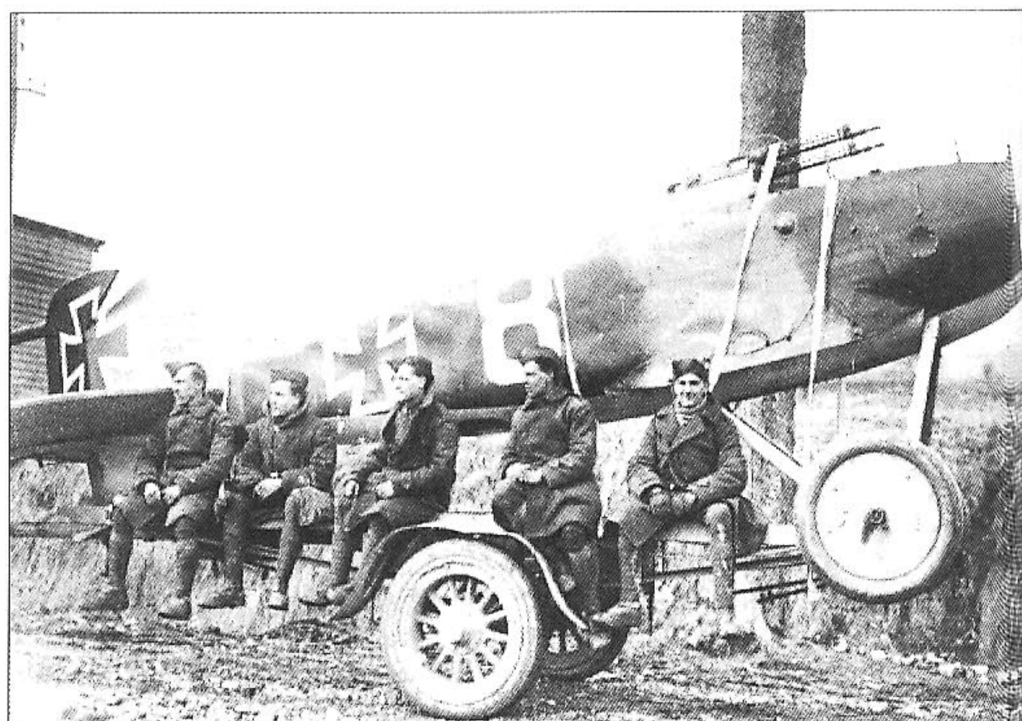
▲ 7 7, 8 and 9. Three of many views taken of Max Böhme's captured Albatros D.II (OAW) 910/16, downed on 3 March 1917. Worth noting are the serial on the wheel disc, the scratched out '4' beneath the '8', the black '8' on the fuselage belly, and the dark band encircling the fuselage just forward of the tail unit.
